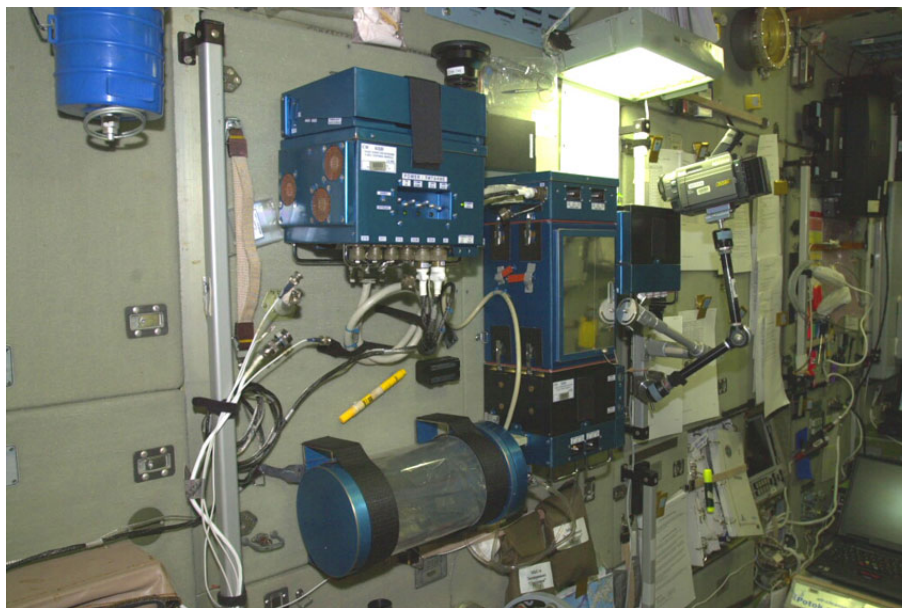
Fig. 1. Greenhouse Lada onboard Russian Segment of ISS
