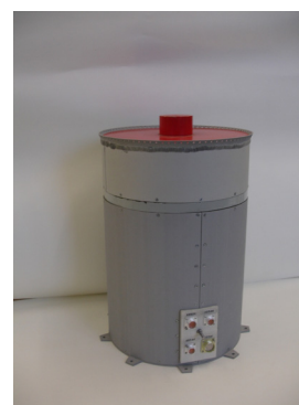
Figure 7. Detector of space dust METEOR-F
