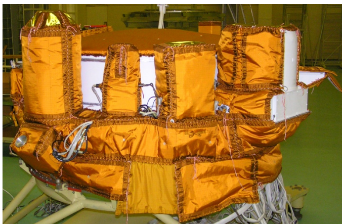
Fig.2. Set of scientific instrument detectors during thermo-vacuum tests in NIIEM.
